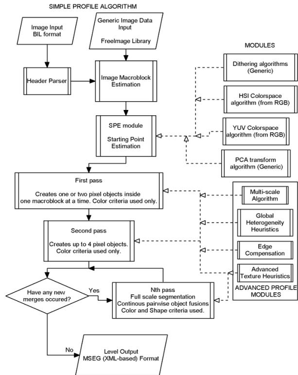
Figure 1: Flowchart of the MSEG algorithm
